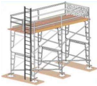
Fabricated Frame / Tubular Welded Frame Scaffold
