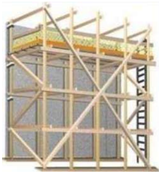
Double Pole Scaffold
